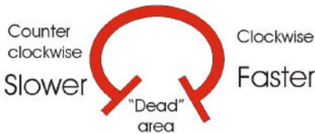
With all pot adjustments, clockwise rotation will increase the cycle speed.
